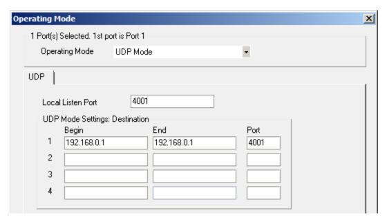
Port 4001 was chosen for the *Local Listen Port*. Data are sent to D2000 KOM process 192.168.0.1, which uses also the local port 4001. We recommend using the same port number within the configuration of one communication line.
