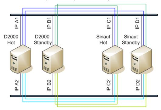
The picture above shows TCP connections - each process D2000 KOM (D2000 Hot, D2000 StandBy) with each Sinaut (Sinaut Hot, Sinaut StandBy)
