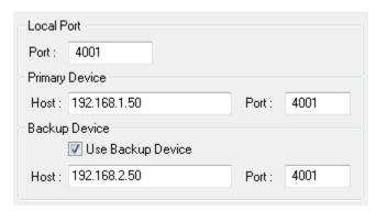
This configuration is completely redundant and resistant to failure of any redundant devices as well as the failure of one of the redundant network segments.
