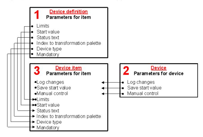
The figure shows the possibilities of the hierarchical definition of values of the configuration parameters, where arrows represent a possibility of inheritance of the parameter and the symbol • represents a possibility (and also place) to define the parameter.
