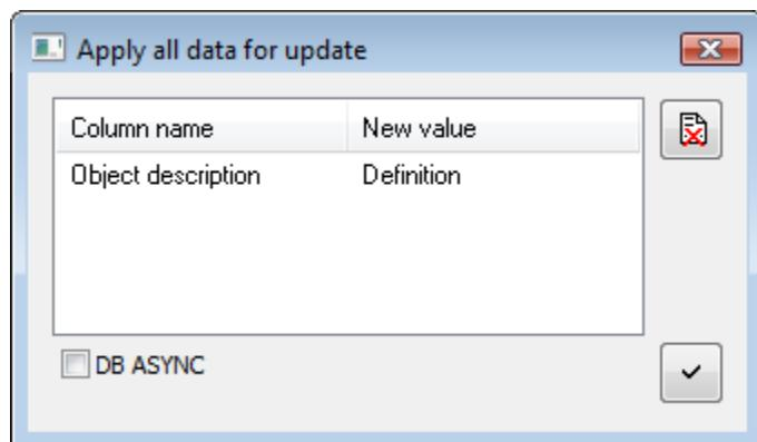
A check box *DB ASYNC* defines whether synchronous or asynchronous record to database is used in the system. Mass update is done after you click on button.
