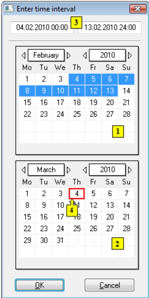
If the function **%History2** is defined for graphic object in picture, the dialog box allows to choose only start time interval (1) and the archived values from the range of one hour from begin of this interval will be displayed.
