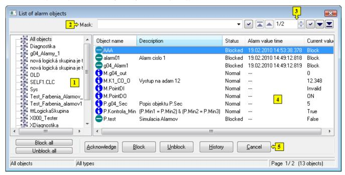
The List of alarm objects window consists of 5 basic parts:
