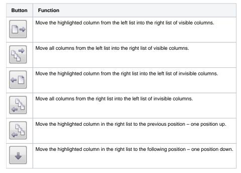
Order of the "Visible columns" (on the right side) determines the order of columns displayed in the dialog box displaying data from the log database. A column placed at the first place will be displayed as the first one from the left, the second column will be the second one from the left, etc.
