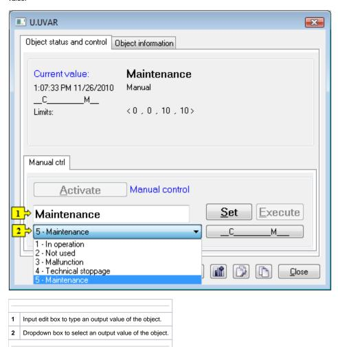
The dropdown box (2) contains the selection of values according to a status text assigned to the object. Predefinition of values for integer and real types of values is described in the following table.
