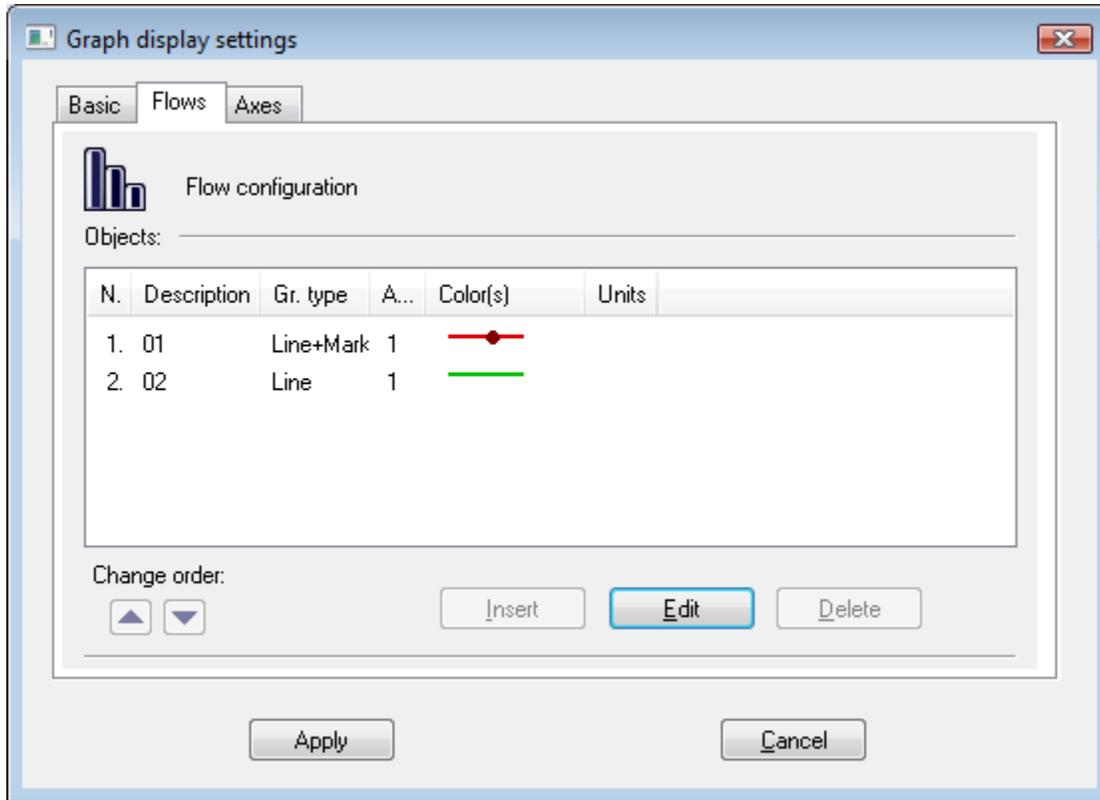
List of flows includes of flow description (the column **Description**) followed by flow type (the column **Gr. type**). The column **Axis** contains the axis number for drawing defined flow. The column **Color(s)** show drawing colors along with additional information (line type, fill, marker, ...). The column **Units** shows defined technical units of corresponding flow (description and technical units will be show in the descriptive table of the XY graph).
