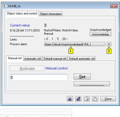
Opens the dialog box to control the given process alarm.
