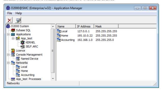
The network is defined by its name, IP address and mask. To define a network, use the following dialog box, which appears when you select **New SubNetwork** from the context menu that is open by right-clicking on **Networks**.
