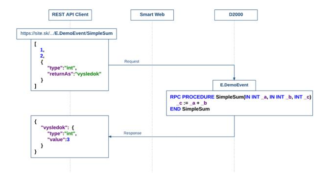
In the figure, there is represented an example of the SimpleSum method calling by a client. The first two parameters are simple JSON types that are implicitly converted to right Unival values. The third parameter is an output one and the client defines in the returnAs attribute the logical name under which will be the output Unival value returned; in this case, it is the logical name "vysledok".
