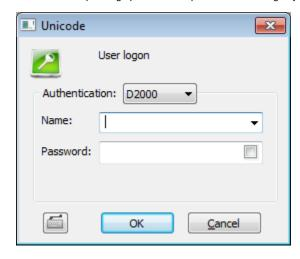
If Enhanced security is a part of your D2000 system licence, the process D2000 HI reads a **logon key** (security token) from the client computer. A logon key is necessary for the user to log on to a D2000 system with *Enhanced security*. The user name is set according to the key which cannot be changed and only password is typed.
