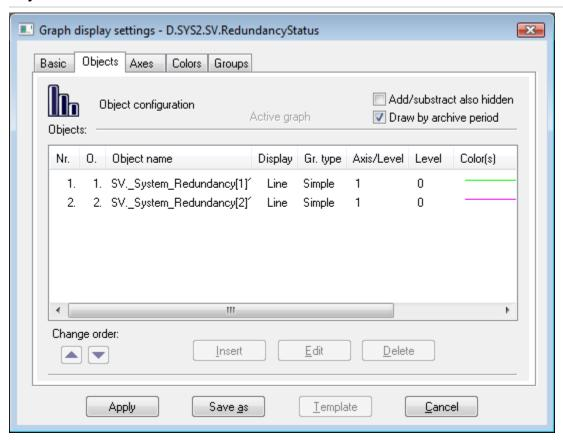
The list of object contains object name followed by graphic flow type with the mark of drawing mode in regard of zero value. Axis/Level column contains the axis number for drawing defined flow and, in case of digital axis, there is also assigned level of the axis. In the column Color(s), there are displayed colors of drawing together with additional information (line type, pattern of flow area filling, selected mark,...).
