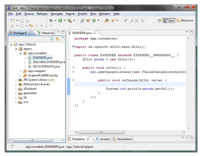
Clicking on the script you can edit it. To save the script in D2000 System you must first save it in Eclipse and then save the object D2000, to which this script belongs, in the D2000 CNF/D2000 GR - the script is loaded from the disc into the D2000 System, compiled, saved into a configuration database and ready to be done.
