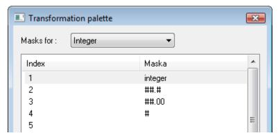
The index of transformation palette is a configuration parameter of specific objects in the system or structures. It determines a representation method of their parameters (using a mask) if this representation is not defined (overloaded) by a linked object of the Status text type, or the linked status text for displayed value is not defined (empty text).
