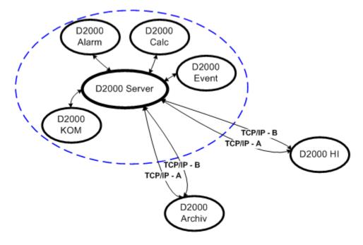
The DUAL TCP/IP technology enables to realize the connection among process D2000 Server and selected (or all) D2000 system client processes via two independent TCP/IP channels. In case of failure of one of the channels, the communication is automatically and transparently rerouted to the other channel.
