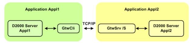
As we can see from the scheme above, there is a communication line between the processes **D2000 GateWay Client** and **D2000 GateWay Server**. This line is used for data transmission between the applications and has been designed to be independent from the versions of the D2000 systems used for the applications.
