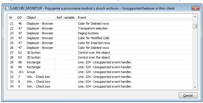
In this dialog window, there is displayed the list of incompatibilities for a picture configuration, from which this window was opened. After clicking the row, the appropriate graphic object will be selected.
