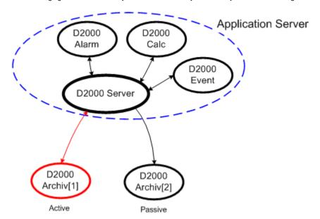
Redundant archiving is realized by increasing the number of the archive processes ( D2000 Archiv) in D2000 system with no need to define them in the DO DM model.
