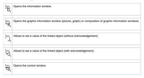
Mouse click on such a graphic object executes the operation corresponding to configuration of the link settings (defined at the picture creation in the process D2000 GrEditor) and linked object type. One of the following operations can be executed:
