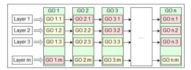
Layer visibility is evaluated during drawing. If layer is visible it will be drawn. Objects are drawn in the layer only if they are defined as visible in this layer.
