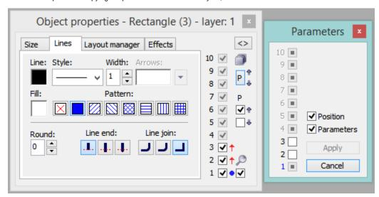
The checkboxes 1 - 10 represents the layers to which data can be copied from the active layer.
