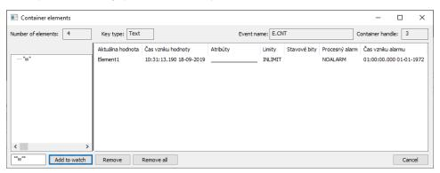
In the left part of the window there are keys of elements of the container, while in the right part of the window there are details of individual elements.
