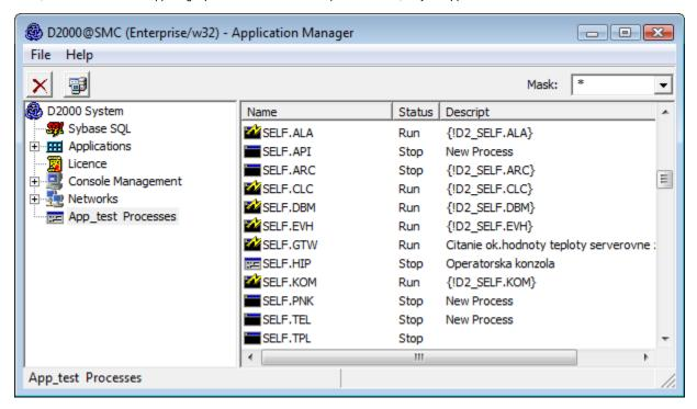
Right-mouse clicking on any process opens the dialog box with one option **Logon** - logon to the process D2000 Server. The process D2000 Server only accepts the logon with administrator access rights. The another right-mouse clicking on any process displays the following pop-up menu:
