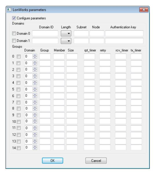
Check Configure parameters if you want to configure the node, otherwise, all the address parameters will not change.
