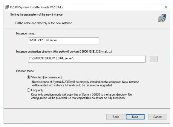
Set the name of the installed instance and the destination directory. Leave the parameter "Creation mode" set as Standard. The given instance name will be used in the *Start menu* after its installation.
