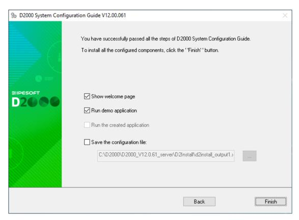
The choice "Run demo application" enables the creating and running of the demo application after the end of the installation. It is possible to save the set parameters of the installation. The last installation phase will run after clicking the button "Finish".
