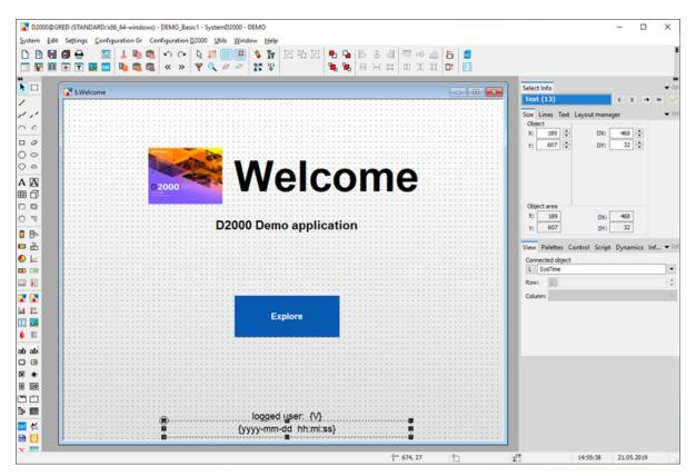
Graphic editor – GR serves for creating visualization and a complete configuration of the application. Currently, it offers configuration of the initial scheme from the previous slide (S.Welcome). If it is changed and saved, the result will be visible in HI (if it is not visible in HI, there is a need to logout and login again).
