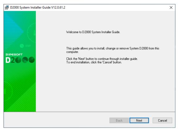
The initial window of the installer guide will open next. It can be controlled by three buttons which enable us to move forward and backward in the dialogue or to cancel the installation altogether.
