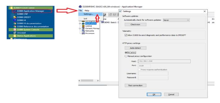
By the choice File/Settings in the Application manager, the Settings window is opened. The correct parameter values of our internet connection can be configured here. The button "Auto-detect" sets everything automatically. If the proxy server is used, the correct parameters of the proxy server must be entered. The correctness of parameters is tested by clicking the button "Test connection".
