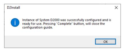
Now the instance of the D2000 system is installed, configured and ready to be used. After clicking the button "Ok", the button "Complete" will be available, shown on the previous slide. By clicking the button, the installation will be completed and the DEMO\_Basic1 application will be created.
