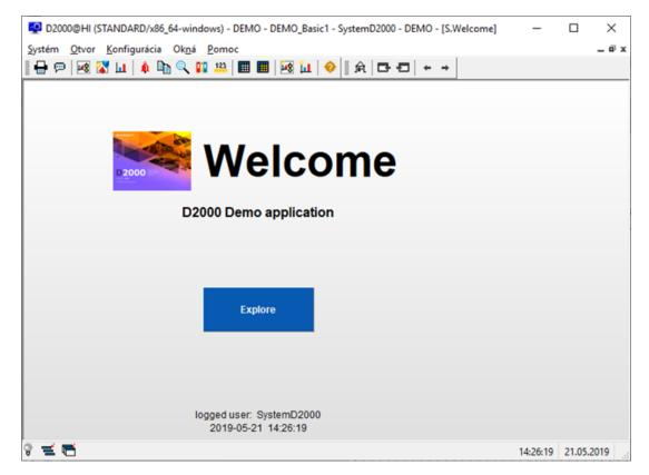
Human Interface – D2000 HI will open with the starting scheme S.Welcome. By clicking on the button "Explore", the main summarizing scheme of the DEMO application will open.
