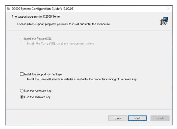
It is necessary to install the PostgreSQL database which is used for storing a configuration of applications. In the case of the Demo version, the support for HW keys, and the choice of the hardware key/software key is not necessary.
