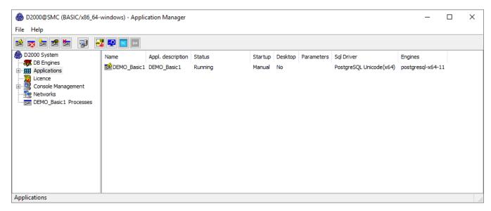
The Application Manager presents the course of creating the DEMO\_Basic1 application and its start. After starting the application, two client processes – HI and GR with the logged-in user SystemD2000 (password: SystemD2000) – will start automatically.
