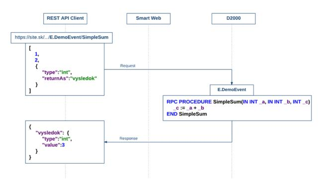
In the figure, there is represented an example of the SimpleSum method calling by a client. The first two parameters are simple JSON types that are implicitly converted to right Unival values. The third parameter is an output one and the client defines in the returnAs attribute the logical name under which will be the output Unival value returned; in this case, it is the logical name "vysledok".
