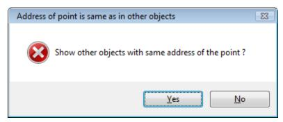
By choosing the option **Yes**, a new CNF dialog window opens. Only I/O tags with conflicting addresses sharing a common parent are displayed in this window. The user can (but does not have to) change the address of these I/O tags.
