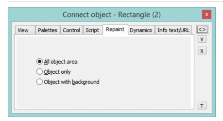
The tab **Repaint** defines a repaint method of the graphic object in the picture after changing the value of connected object. It also defines how to repaint it while blinking. The tab contains the following options.
