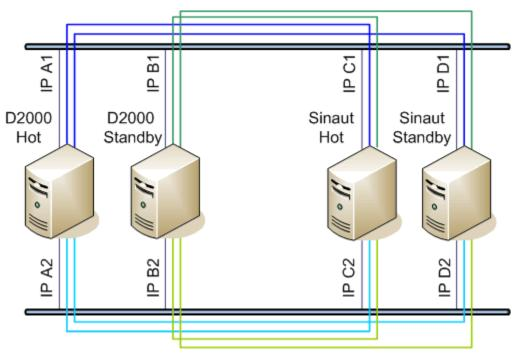
Picture: the D2000 redundant system communicating with Sinaut redundant system in a redundant network
