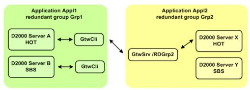
D2000 GateWay Server is started on every application server in redundant group Grp2 (with the start parameter /S or without it if it runs on the same computer as D2000 Server). In this mode D2000 GateWay Server disconnects D2000 GateWay Client if the server D2000 GateWay Server is connected to is not HOT.
