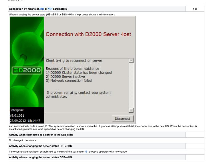
If the connection has been established by means of the parameter /S, process operates with no change.
