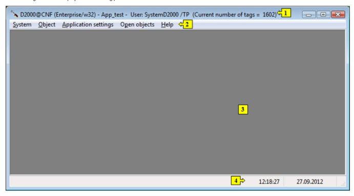
The environment of process D2000 CNF comprises of the following basic parts:
