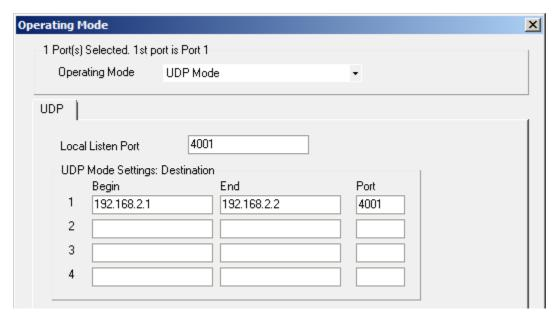
The above-mentioned settings show that both NPort devices send data to both D2000 servers (i.e. KOM processes), to IP addresses in that network in which it is connected (NPort 1 in Ethernet A and NPort 2 in Ethernet B).
