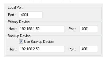
This configuration is completely redundant and resistant to failure of any redundant devices as well as the failure of one of the redundant network segments.
