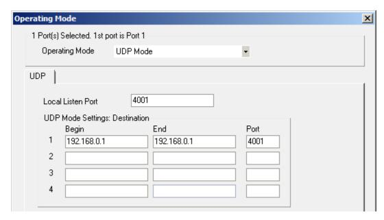
The port 4001 was chosen for *Local Listen Port*. Data are sent to D2000 KOM process 192.168.0.1, which uses also the local port 4001. We recommend to use the same port number within the configuration of one communication line.
