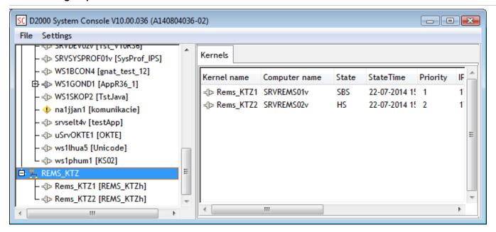
Text console contains the only tab - Kernels. It shows the list of servers included in the redundant group.
