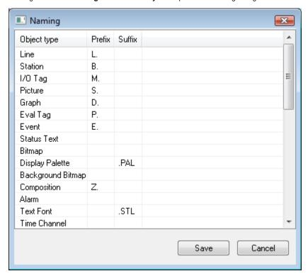
The dialog box includes the list of individual object types as well as some specific objects (e.g. object representing the start and stop condition of system alarms, start object (trigger) for events etc.).
