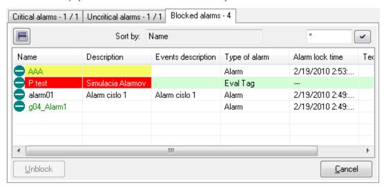
The tab name comprises its name and the number of blocked alarms in the system. The button activates the basic sorting of the list by the first column. The parameter **Sort by** shows the current order of the list. Beside the parameter, there is the input field for entering a mask for selecting objects by entered name.
