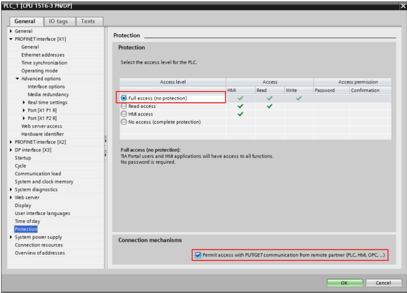
V prípade TIA Portal verzie 14 je nastavenie "Permit access with PUT/GET communications from remote partner" na samostatnej záložke "Connection mechanisms" pod "Protection & Security":
