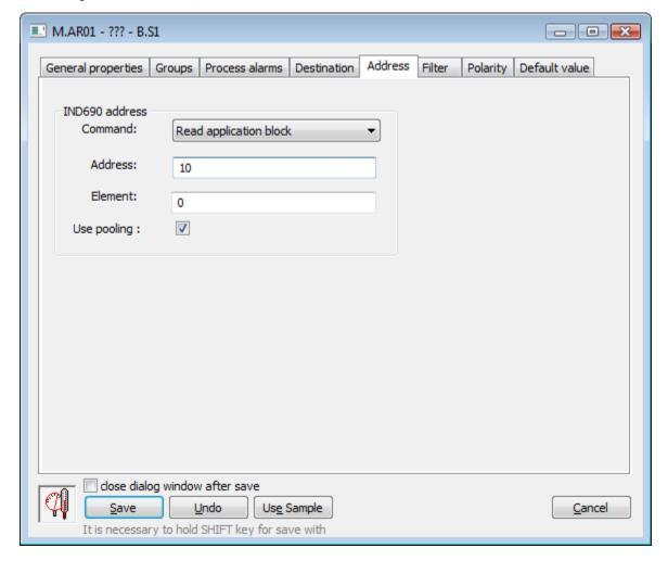
I/O tag address consists of three basic parts:
