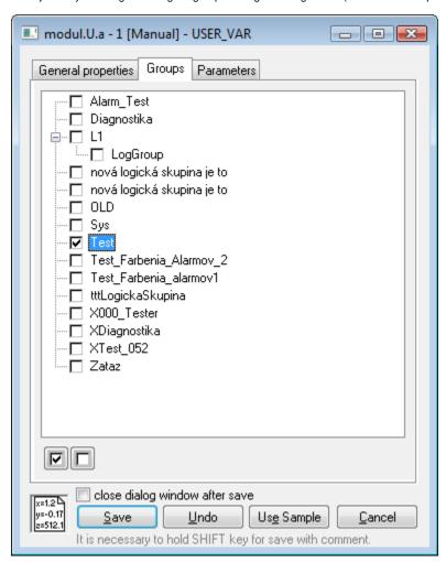
The tab contents is formed by the tree structure of all logical groups defined in the application. The symbol in front of the name of each group shows if a configured object is or is not a member of the particular group. It may be changed by left-clicking a particular symbol.
