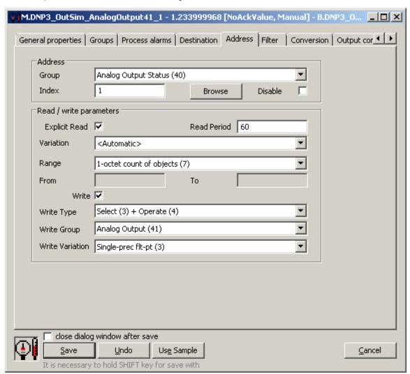
Figure - the configuration of I/O tag address for DNP3 protocol
