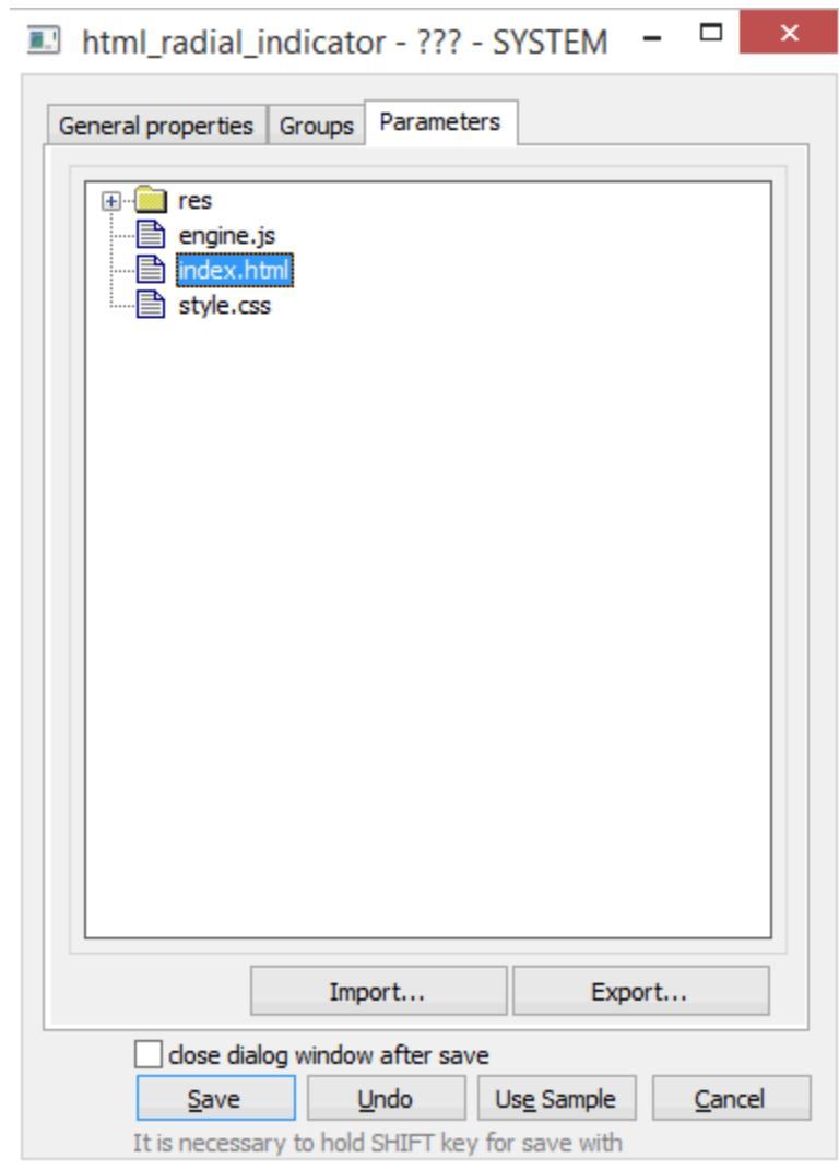
User may insert the files or directories by clicking the **Import** button, or by drag-and-drop from the windows explorer or other application. The **Export** button allows saving files onto the disk.
