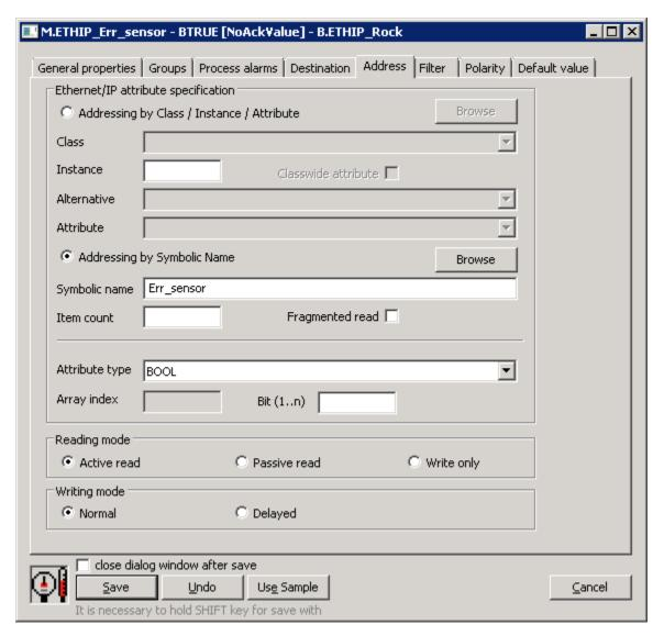
This addressing method is supported by Rockwell devices. It uses Proprietary Rockwell messages:
