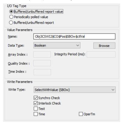
Write type - the type of writing. IEC-61850 defines 4 write models (IEC 61850-7-2):
