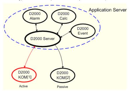
Redundancy of communication process is realized by increasing the number of the communication processes (D2000 KOM) in system without the need to define them in the DODM model.
